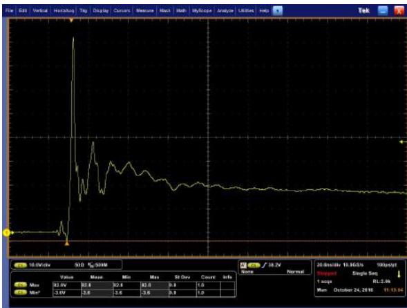
Fig 3 .Positive 8kV contact per IEC61000-4-2
