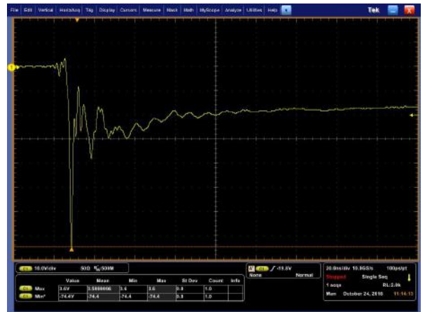
Fig 4 .Negative 8kV contact per IEC61000-4-2
