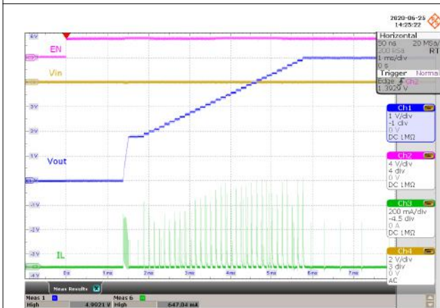
Figure 8-28. Start-up Behavior from Rising Enable
