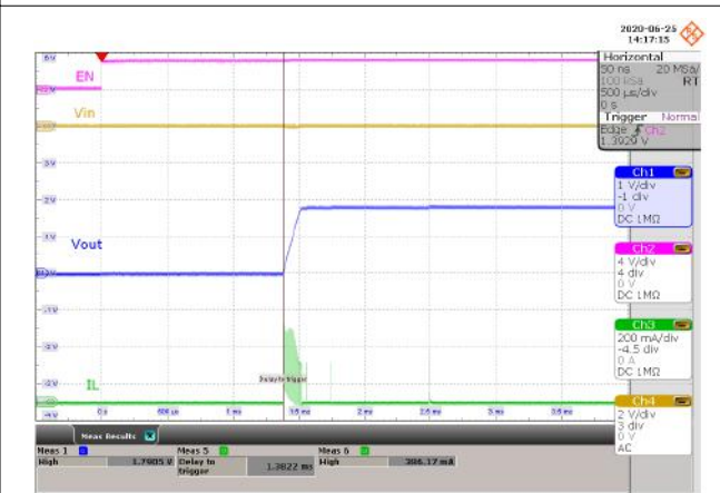
Figure 8-27. Load Transient, 300 mA Step
