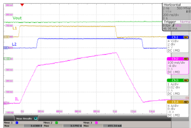
Figure 8-11. Switching Waveforms, Boost Operation
